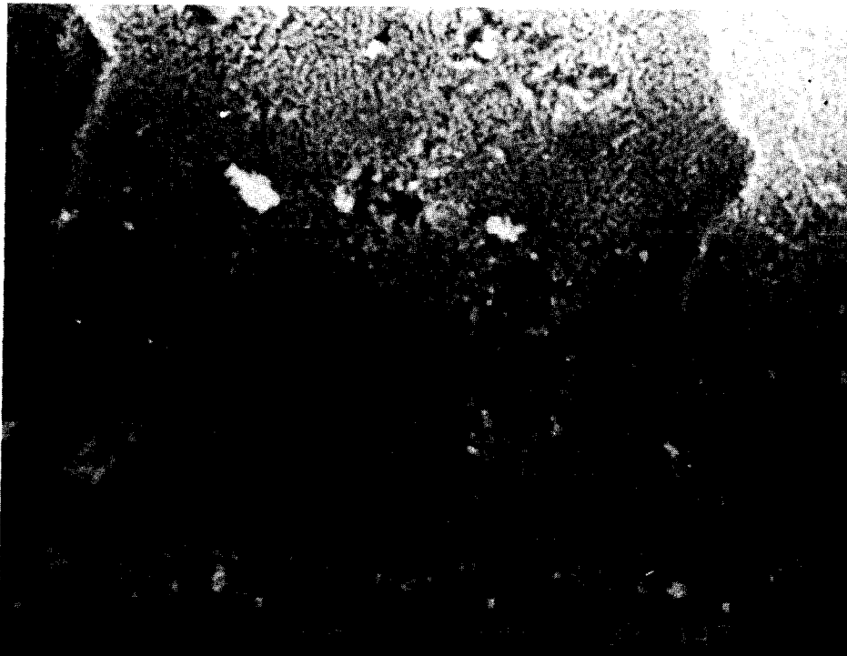
FIG. 14. Single particle of the fresh Raney Cu catalyst, with pore structure visible (SEM).
